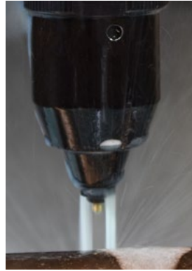
With high pressure internal coolant
