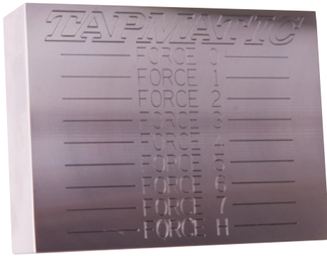
Example in 4140 pre heat treated material with hardness 28 HRC. Marking at different settings with 1.3 mm compression against the surface.
