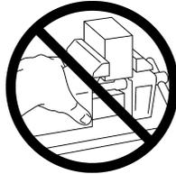
The tapping attachment can become hot to the touch after operation. Use caution when removing from the machine or handling.
