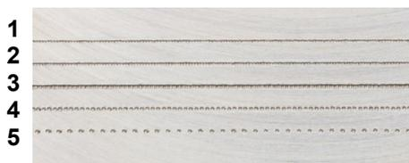
1. Marking plane 3mm, 750 RPM, 250 mm/min.
