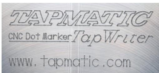
Marking plane 3mm, 850 RPM,
