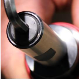
Remove cap with 5mm hex key.
