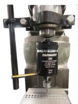
Always mount a torque bar to hold the tapping attachments stop arm from rotating. The torque bar **must** be mounted securely to the table or quill of your machine. The torque bar installation must be stronger than the largest tap in the capacity range of your tapping attachment. The surface of the torque bar must be smooth to allow the stop arm to slide freely when feeding in and out of the hole. Order Tapmatic Torque Bars shown.
