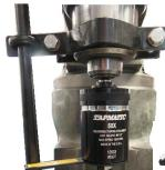
Always mount a torque bar to hold the tapping attachments stop arm from rotating. The torque bar must be mounted securely to the table or quill of your machine. The torque bar installation must be stronger than the largest tap in the capacity range of your tapping attachment. The surface of the torque bar must be smooth to allow the stop arm to slide freely when feeding in and out of the hole. Order Tapmatic Torque Bars shown.
