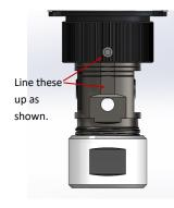
Hard Start: Use this position for more accurate depth control. Turn the collar until it just contacts the bottom of the housing/gear carrier. Push up against the Rubber Flex spindle and it should not compress. Self Feed for tapping in this position is... 30TC/DC approx. 3mm 50TC/DC approx. 6mm
