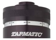
Clutch adjustwhen tapping blind holes. Tightening the cap down to the higher number settings on the reference scale increases torque. To set the torque, use a new tap and begin with a low number (low torque) setting. Try to tap the hole.
