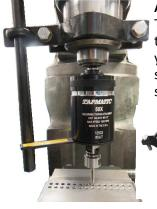
Always mount a torque bar to hold the tapping attachments stop arm from rotating. The torque bar **must** be mounted securely to the table or quill of your machine. The torque bar installation must be stronger than the largest tap in the capacity range of your tapping attachment. The surface of the torque bar **must be smooth** to allow the stop arm to slide freely when feeding in and out of the hole. Order Tapmatic Torque Bars
